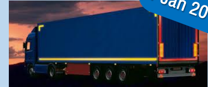
Retro-Reflective Installation (UN R104)
