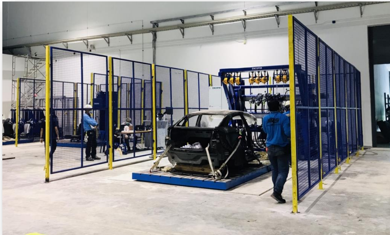
Seat Belts Anchorages test system
