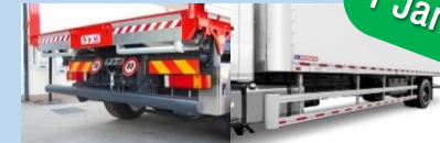
Lateral and Rear Underrun protective devices RUPD, LPD (UN R58, 73)
